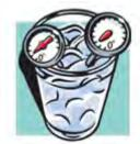
2. Set the probe of the thermometer in the mixture, making certain it's not touching the sides or the bottom. Wait until the needle stops moving to see what temperature it's reading. If it's not 0°C (32°F), it needs to be adjusted.
