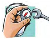
3. If your thermometer has a calibration nut, use a small wrench to turn it until the temperature reads 0°C (32°F). Keep the probe in the ice water to make sure the temperature is accurate.
